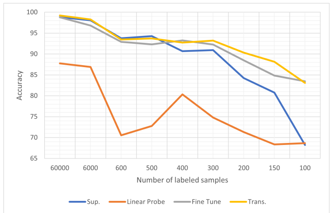
Fig. 2. Model performance. Classification accuracy against the number of labelled images used for training. Performance for models initialized with a self-supervised model (Linear Probe, Fine Tune and Trans.) decrease slower than the fully supervised model (Sup.).
