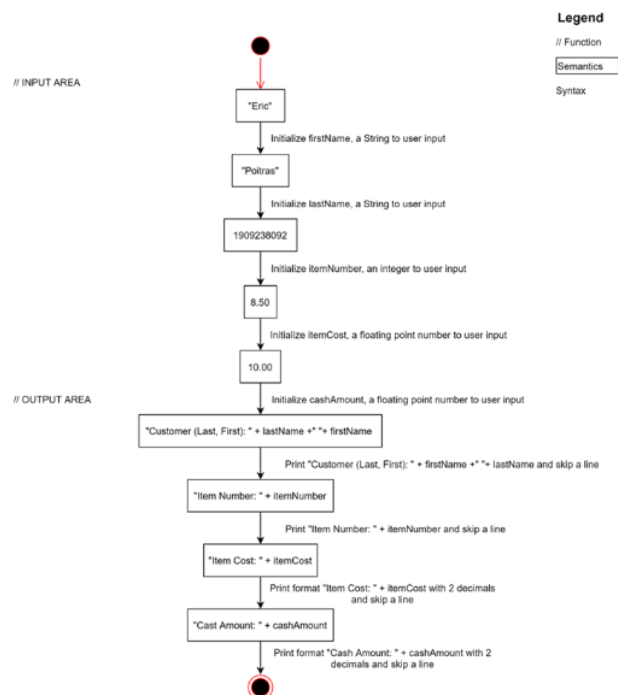
Figure 1: An example flow diagram including pseudocode and trace depictions of operations designed as a solution to a programming problem.
